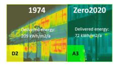
In the zero2020 building (which contains NBERT), the energy system is composed of an **air to water heat pump**, **low temperature radiators**. Moreover, a **micro-grid** powers the building while also exporting energy to the national grid. The improvements in the buildings fabric is clear above. This was also shown the building energy ratings achieved after the retrofit.
